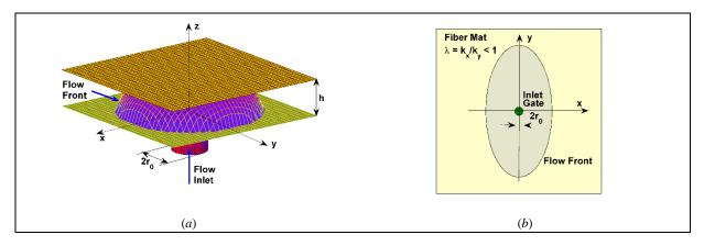
Figure 1: Physical models for transverse (a) and in-plane (b) permeability measurements showing the inlet gate and the front of the fluid injected through the fiber matrix.
